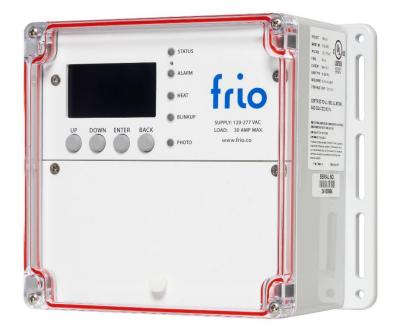
The S1 is a single-circuit IoT heat trace controller for use in snow melting, freeze protection and temperature maintenance applications. The device can drive up to a 30A resistive load to control electric heat trace systems operating between 120 VAC and 277 VAC. The S1 comes in an outdoor-rated enclosure tested to IP67 & NEMA 4X standards.
